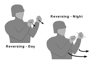
Fist at chest level during the day and chemlights in fist pointing at each other at night. This signal is given with a pumping action to signal reversing.
