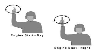
Hand or chemlight at head level moved in a circular motion signals "START ENGINE"
