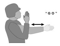
The hand will be extended from the chest toward aircraft opening to indicate "GO" for all roping & casting operations.
