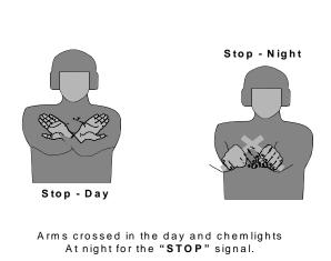
Figure 12-3. Stop Load Signal.
