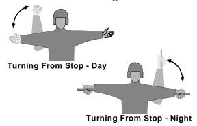
The signal arm will be held in the vertical position during the day and chemlight at night moved in a pumping motion. The other arm/chemlight will be pointed in the direction the tires need to be turned. This signal is given to a stopped vehicle.
