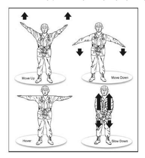
Figure A-1. Hand Signals for Directing Aircraft Movement.
