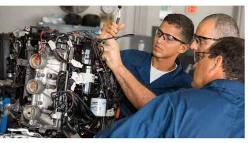
Outboard Motor Maintenance and Overhaul (OBM) is an eight-week course of instruction designed to provide Foreign Security Force personnel with the knowledge and skills required of a basic outboard motor technician.
