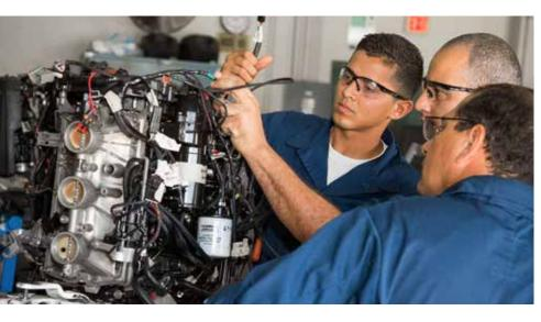
Outboard Motor Maintenance and Overhaul (OBM) is a seven-week course of instruction designed to provide Foreign Security Force personnel with the knowledge and skills required of a basic outboard motor technician.
