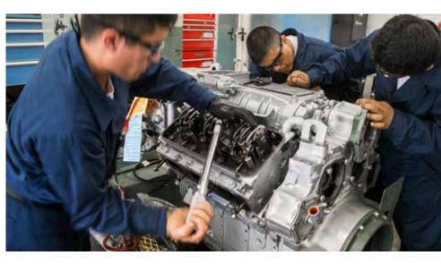
Diesel Systems Overhaul and Maintenance (DSOM) is a seven-week course of instruction designed to provide Foreign Security Force personnel with the knowledge and skills required of a basic diesel engine technician.
