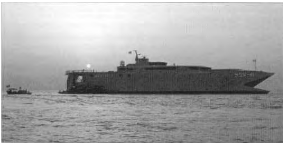
The high speed vessel Joint Venture, a 315 foot-long, aluminum-hull catamaran that has been modified to carry gunboats, amphibious landing craft, helicopters and marine platoons, became a seaborne forward operating base for Navy SOF, who helped to clear southern Iraqi waterways of Iraqi ships and mines. (Photo by Petty Officer 1st Class Arlo K. Abrahamson)
