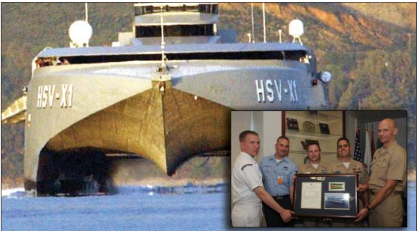
(Main photo) The multi-service high-speed vessel, Joint Venture (HSV-X1) is a 313-foot-long experimental craft and is a wave-piercing catamaran capable of 45 knots. Photo by Paul Farley. (Bottom right) Former crew members of the Joint Venture (HSV-X1) hold a framed certificate of the Meritorious Unit Commendation medal. The crew was recognized for providing support to Special Operations Forces and giving humanitarian assistance to countries throughout Southeast Asia. Photo by Petty Officer 2nd Class Shauntae Hinkle.
