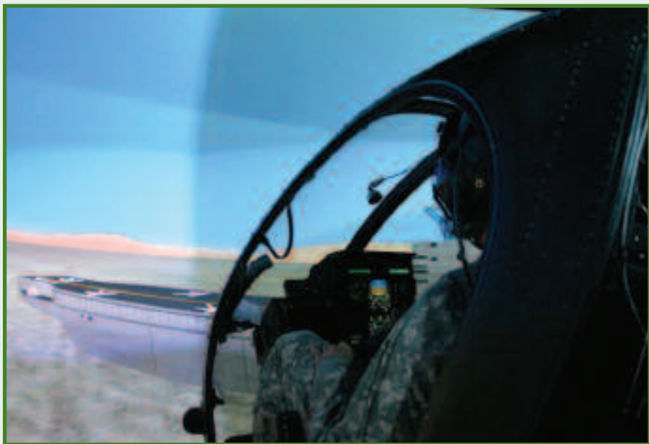
The 160th Special Operations Aviation Regiment (Airborne) MH-6M combat mission simulator utilizes an MH-6C airframe. Courtesy photo.
