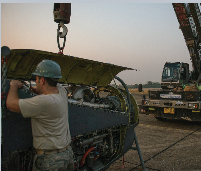
Members of the 353rd Special Operations Maintenance Squadron perform an engine change for an MC-130H at exercise Cobra Gold, in Udon Thani, Thailand, Feb. 14. The 353rd SOMXS's mission is to organize, train and equip Airmen to perform aircraft maintenance and back shop support for the MC-130H flown by the 1st Special Operations Squadron as well as other special operations aircraft.
