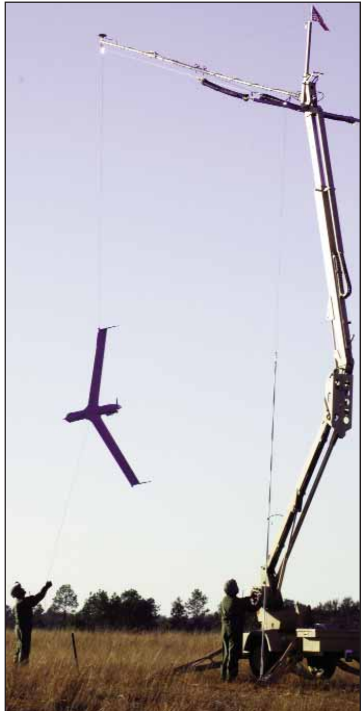
Airmen from Moody Air Force Base, Ga., lower the Scan Eagle unmanned aircraft system after it was recovered by the Skyhook system during a demonstration to highlight its capabilities at Eglin AFB, Fla. AFSOC is the lead command for SUAS and has been working with the team to prepare and certify Scan Eagles to employ the system in the near future. Photo by Senior Airman Emily Moore.
