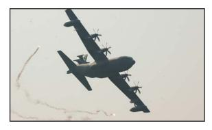
The **EC-130E/J Commando Solo**, a specially-modified fourengine Hercules transport, conducts Information Operations, Psychological Operations and Civil Affairs broadcasts in AM, FM, HF, TV and military communications bands. A typical mission consists of the Commando Solo flying near and broadcasting to the desired audience – either military or civilian personnel.
