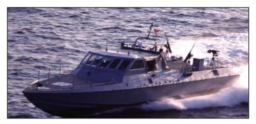
The Special MK V Operations Craft performs medium-range infiltration and extraction of SOF, limited coastal patrol and interdiction in low to medium threat environments. The MK V SOC is a high performance combatant craft sized to permit air deployment aboard C-5 aircraft. Each craft is manned by a crew of five Special Warfare Combatantcraft Crewmen and can carry 16 SOF personnel.
