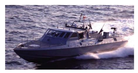
The Mark V Special Operations Craft performs medium-range infiltration and extraction of SOF, limited coastal patrol and interdiction in low to medium threat environments. The Mark V SOC is a high performance combatant craft sized to permit air deployment aboard C-5 aircraft when mated to organic transporter and in company with other support equipment. Each craft is manned by a crew of five Special Warfare Combatant-craft Crewmen and can carry 16 SOF personnel.
