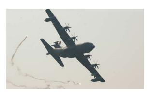
The **EC-130E/J Commando Solo**, a specially-modified fourengine Hercules transport, conducts Information Operations, Psychological Operations and Civil Affairs broadcasts in AM, FM, HF, TV and military communications bands. A typical mission consists of a single-ship orbit offset from the desired target audience – either military or civilian personnel.
