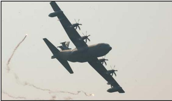
The **EC-130E/J Commando Solo**, a specially-modified four-engine Hercules transport, conducts Information Operations, Psychological Operations and Civil Affairs broadcasts in AM, FM, HF, TV and military communications bands. A typical mission consists of the Commando Solo flying near and broadcasting to the desired audience – either military or civilian personnel.
